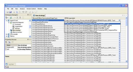
The left column contains a list of all of the AutoShape types the plugin can recognize.
